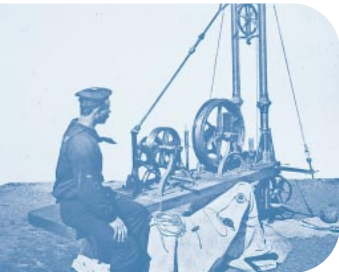
The Sigsbee sounding machine for measuring bottom depth during a 1904 cruise aboard the U.S. Fisheries steamer Albatross.
